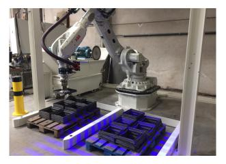
One of the key technologies is the use of ABB's Integrated Force Control which allows speed or pressure control. Normally robots are position controlled with a predefined path and speed. With the Integrated Force Control, the robot reacts to its surroundings and deviates from the programmed path or speed based on feedback from the force sensor. The adapted movement of the robot is determined by constraints that are specified to suit the particular application.
